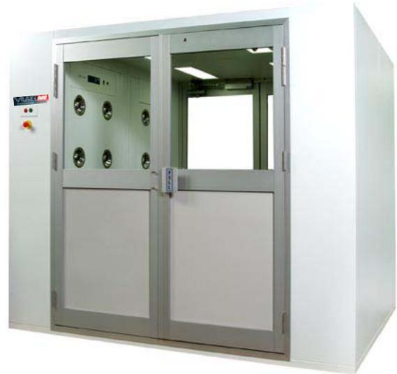
**Two-Way One-Way:** Only one door at a time can be opened. Both doors are unlocked at rest. Person enters door at cleanroom exterior. Air shower cycle starts. At end of cycle person exits via door at cleanroom interior. Alternatively, person can enter via door at cleanroom interior, proceed through unit and exit via door at cleanroom exterior without initiating the fans.
